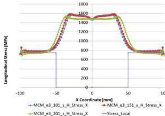
Analytical solution and the SPH-experiment 3 numerical results for longitudinal stress at  $t = 3/2 \cdot L/c_e$
