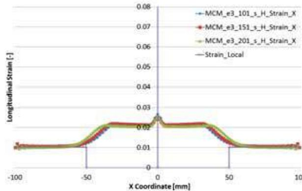
Analytical solution and the SPH-experiment 3 numerical results for longitudinal strain at  $t = 3/2 \cdot L/c_e$
