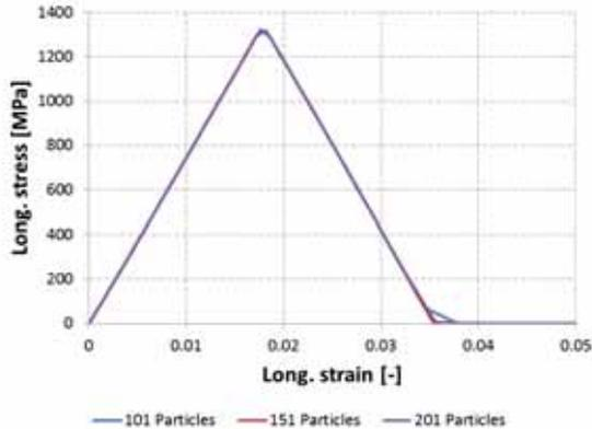
Longitudinal stress vs. longitudinal strain curves for the central particle for different values of  $\Delta p$ , SPH
