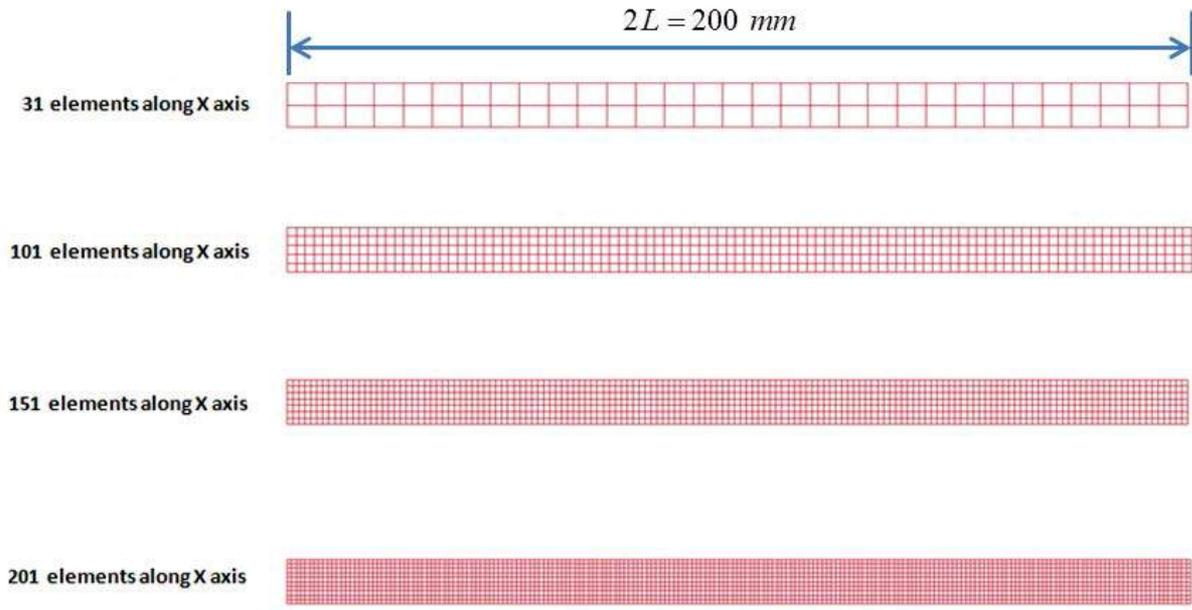
**Particle discretisation in SPH (MCM) of strain-softening bar**
