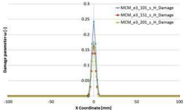
Damage distribution for different particle densities, SPH-experiment 3, response time  $t = 3/2 \cdot L/c_e$
