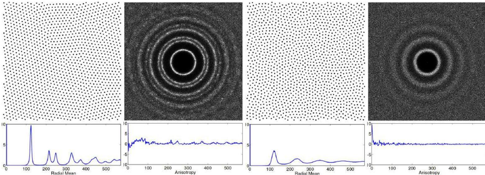
**Effective Nyquist Frequency:** size of “flat spot” **Oscillation:** magnitude of ripples<sup>4</sup>
