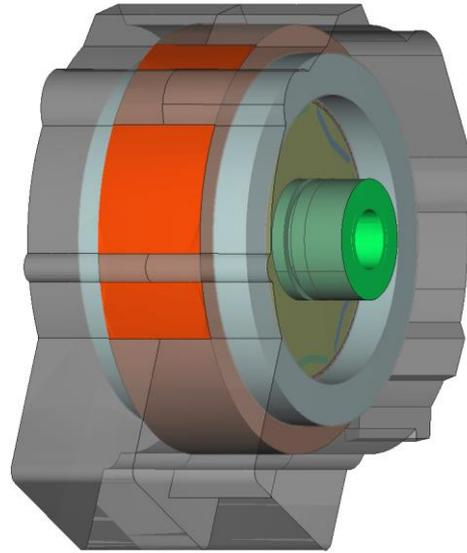
Oil flow through rotor shaft
