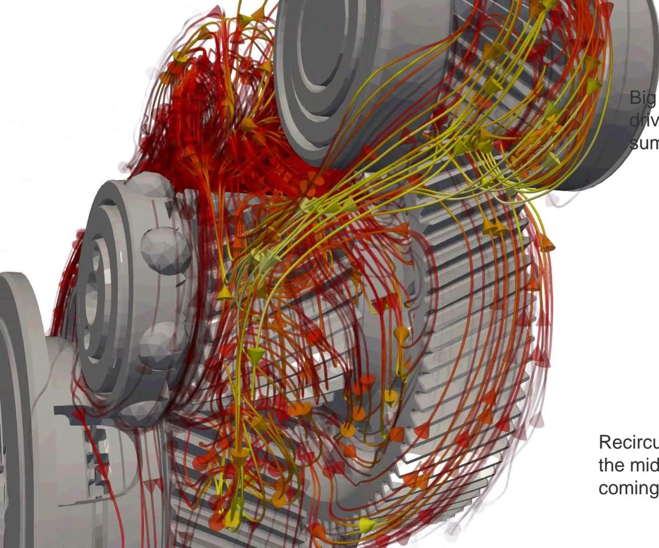
Big gear on the middle shaft drives the oil back into the main sump.
