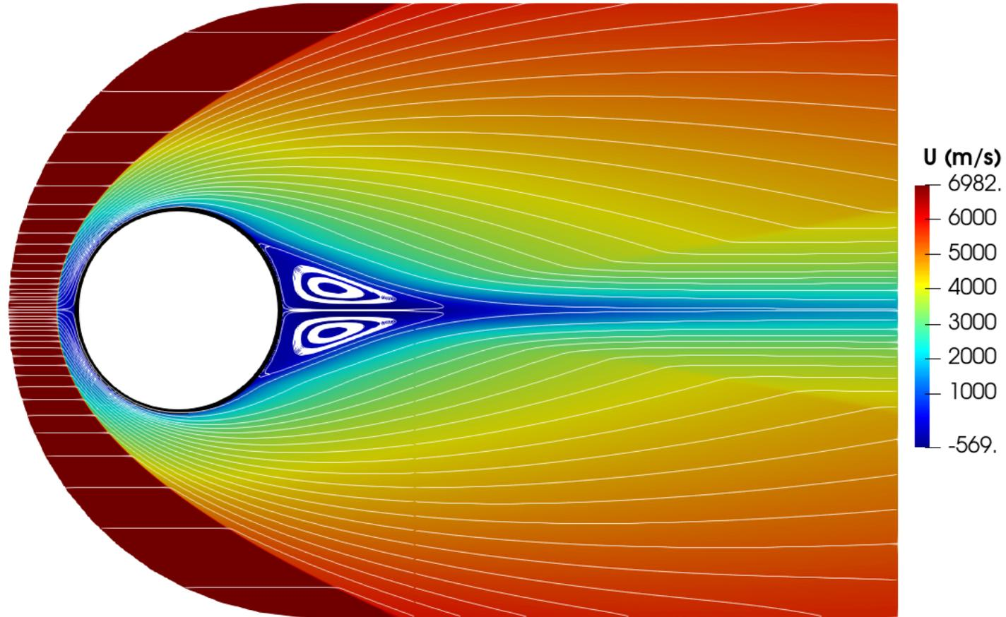
Typical features associated with a high-Ma, continuum flow like a 'thin' shock, wake-recirculation region, downstream re-compression shock etc. captured.
