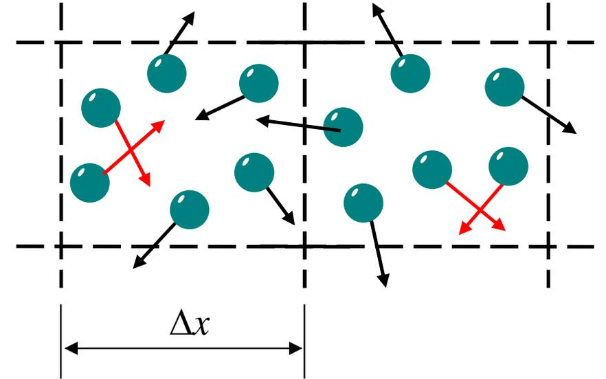
To ensure accuracy,  $\Delta x$  and  $\Delta t$  need to be less than mean free path & mean free time respectively.
