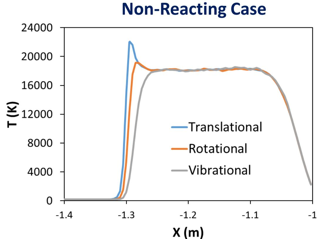
Shock structure, shock standoff distance and Temperature components significantly different if chemical reactions are ignored.
