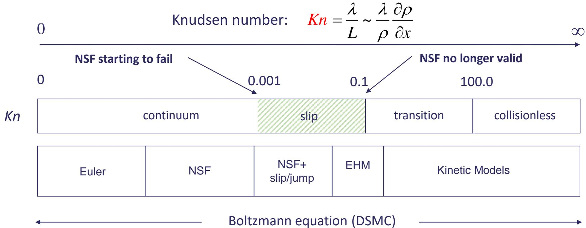
**Key Message:** Molecular (Kinetic) level methods like DSMC needed, in situations where traditional CFD is invalid. Example applications: *high-altitude hypersonics*, *vacuum gas dynamics* and *micro-nanofluidics*.
