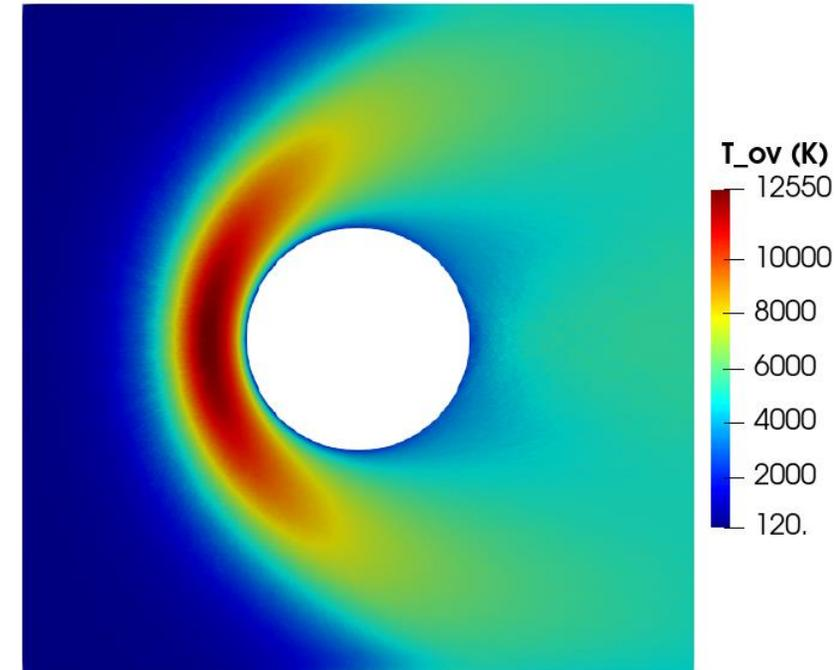
Flow rarefaction significantly affects the shock structure and shock standoff distance.
